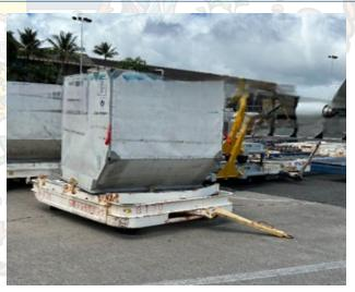
Front ULD shows tow bar in the "down" position – brake not activated. Rear ULDs in the background show proper "up" position – brake activated. (above photo)
