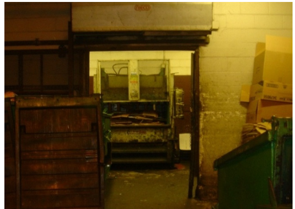
Figure 9. Example of a concession owned cardboard baler which typically compact 20 lbs. of cardboard per cubic foot of baled material.
